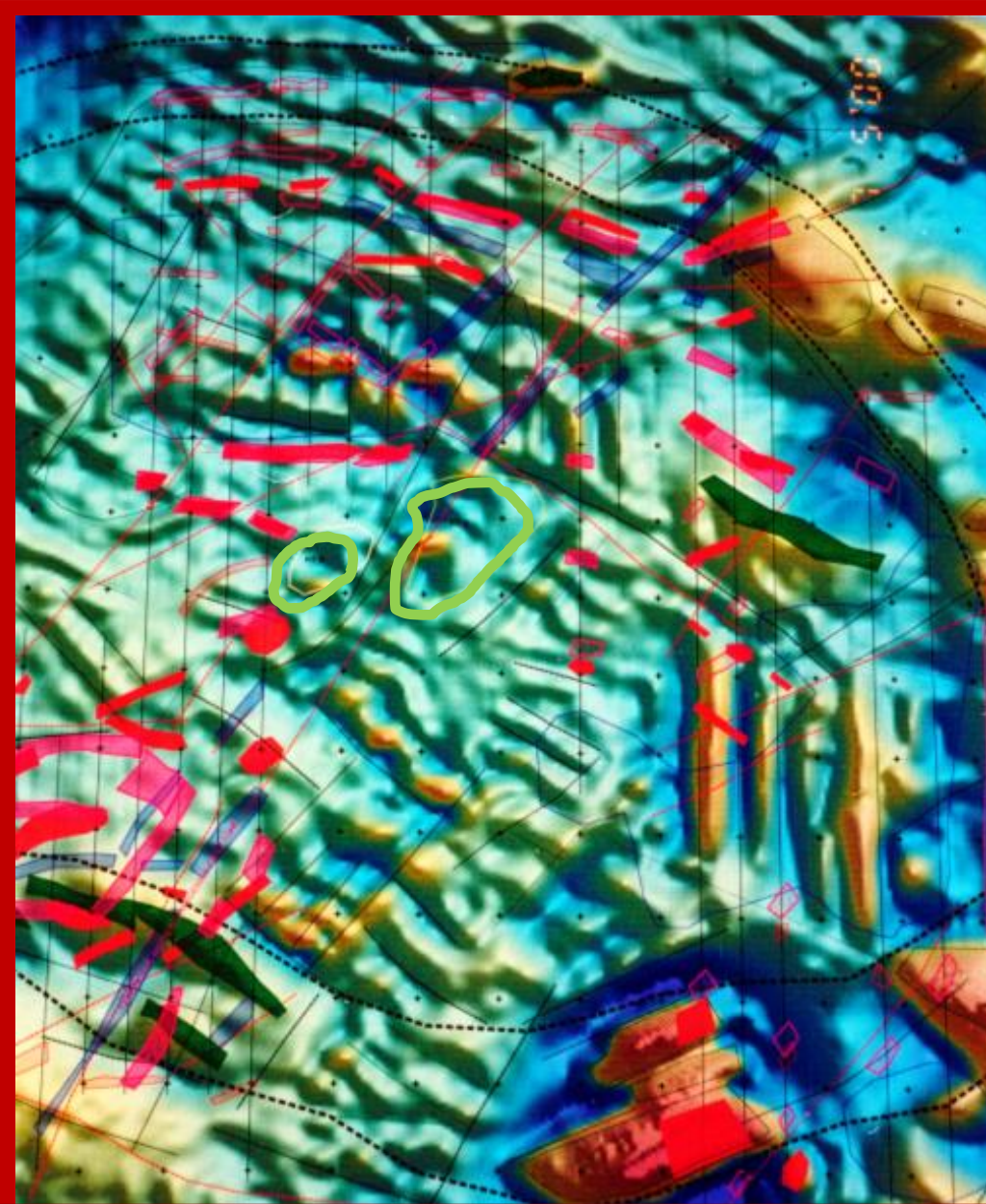
The OreFull Mineral Texture Atlases Volume 48 – 2 : North Queensland Epithermals WIRRALIE - Regional Magnetics Shaded RTP on Dipole Dipole Resistivity. Pits A and B in green and possible targets in red (left side). Resistivity is on the right side. Data with permission from Delta Gold and initially generated by Dr. Greg Partington and Team .
